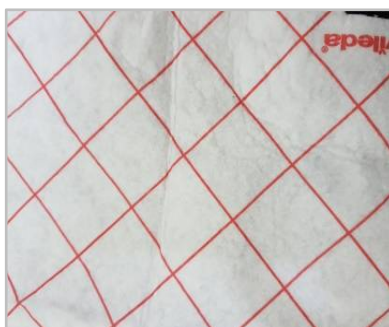
Figure 2. Fibrous texture as separator in supercapacitors.
