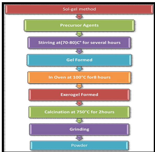
Figure 2. A block diagram for preparation of powder by sol-gel method.
